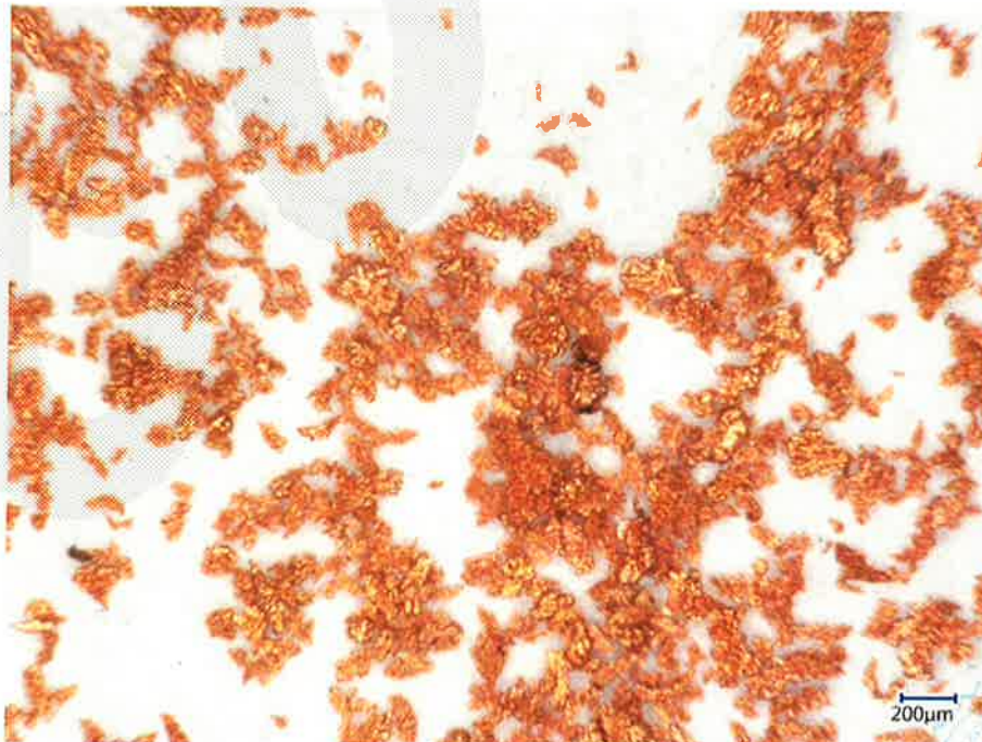
Figure 2: Light microscope image of the "copper powders", x200
